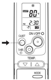
QUIET Mode is used to reduce the fan sound of the indoor unit.
